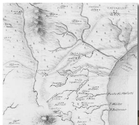
Detail of Schiantarelli's map of the 1783 Calabrian earthquake - different symbols are used for villages according to the amount of damage
