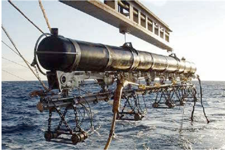
seismische Exploration (airgun array)
